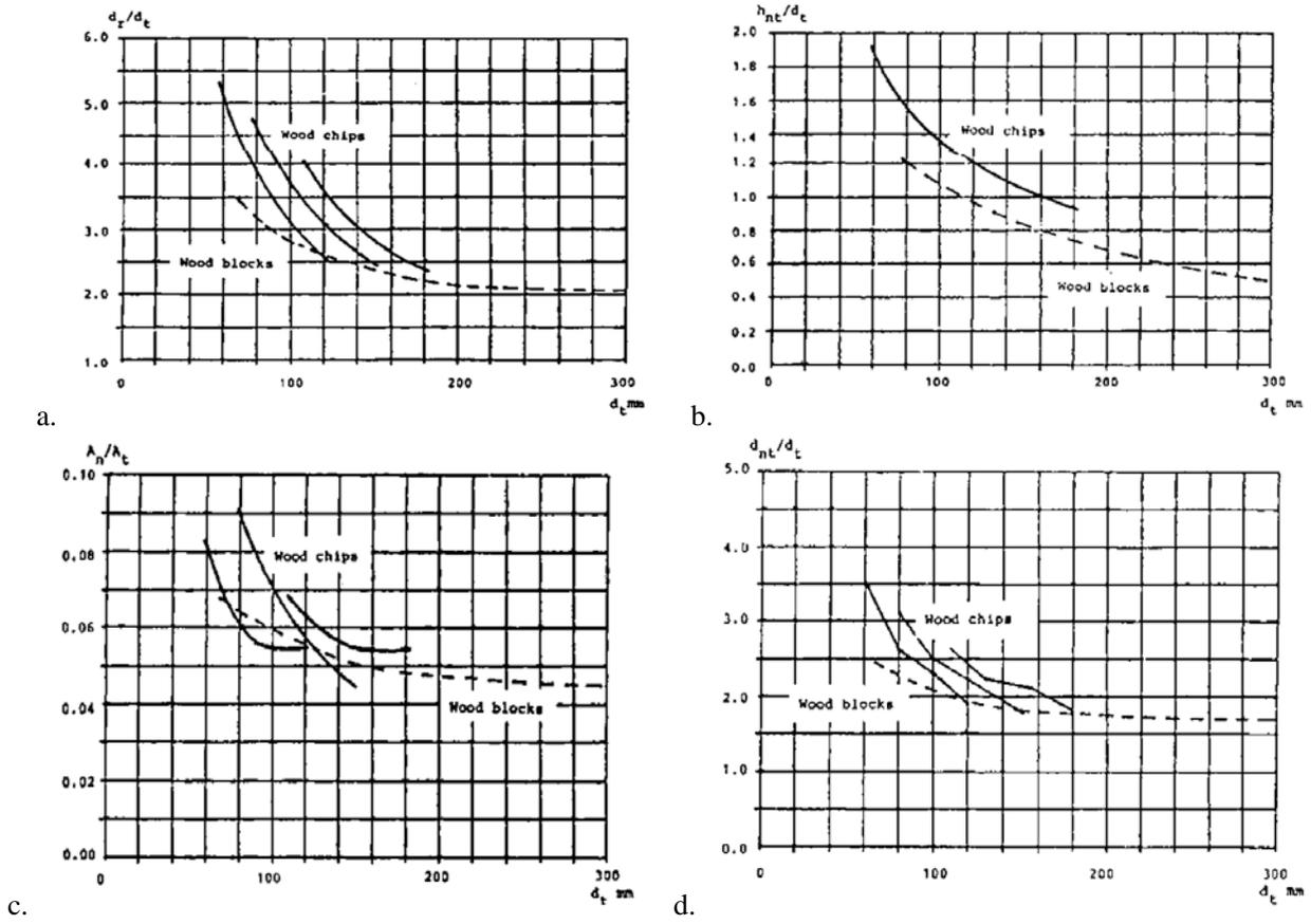
Fig. 1 a. Diameter of the fire box,  $d_f$ , as a function of the throat diameter,  $d_t$ ; b. Height of the nozzle plane above the throat,  $h_{nt}$ , as a function of the throat diameter; c. Ratio between nozzle flow area,  $A_n$ , and throat area,  $A_t$ , as a function of the throat diameter; d. Nozzle tip ring diameter,  $d_{nt}$ , as a function of the throat diameter,  $d_t$  [1].
