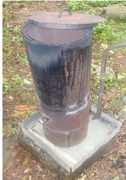
Fig. 3 The laboratory scale biomass gasifier.
