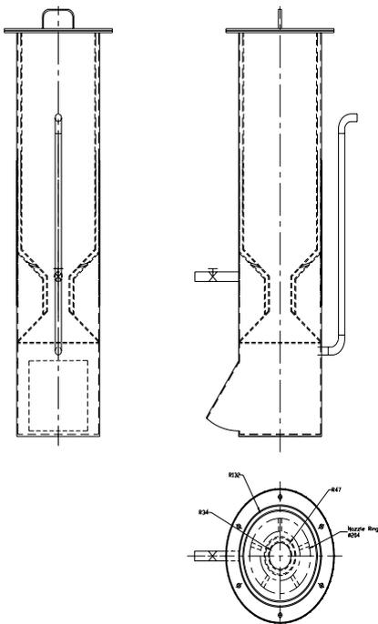
Fig. 2 Orthographic views of the laboratory scale biomass gasifier.
