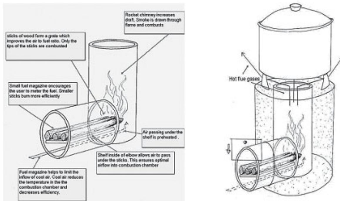
**Figure 24:** Diagrams showing the principles behind the fuel efficiency in rocket stoves\_Sengratry/ Winiarski Buekens\_1990
