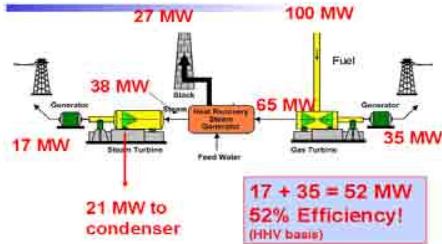
Figure 29 Gasification for power generation\_Sengratry/Steve Jenkins\_2005
