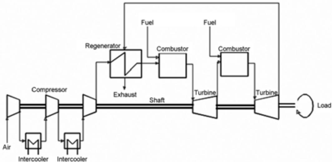
**Figure 28: Gas turbine with heat recovery, intercooling and reheat\_Sengratry/ Gary J.Stiegel\_2005**
