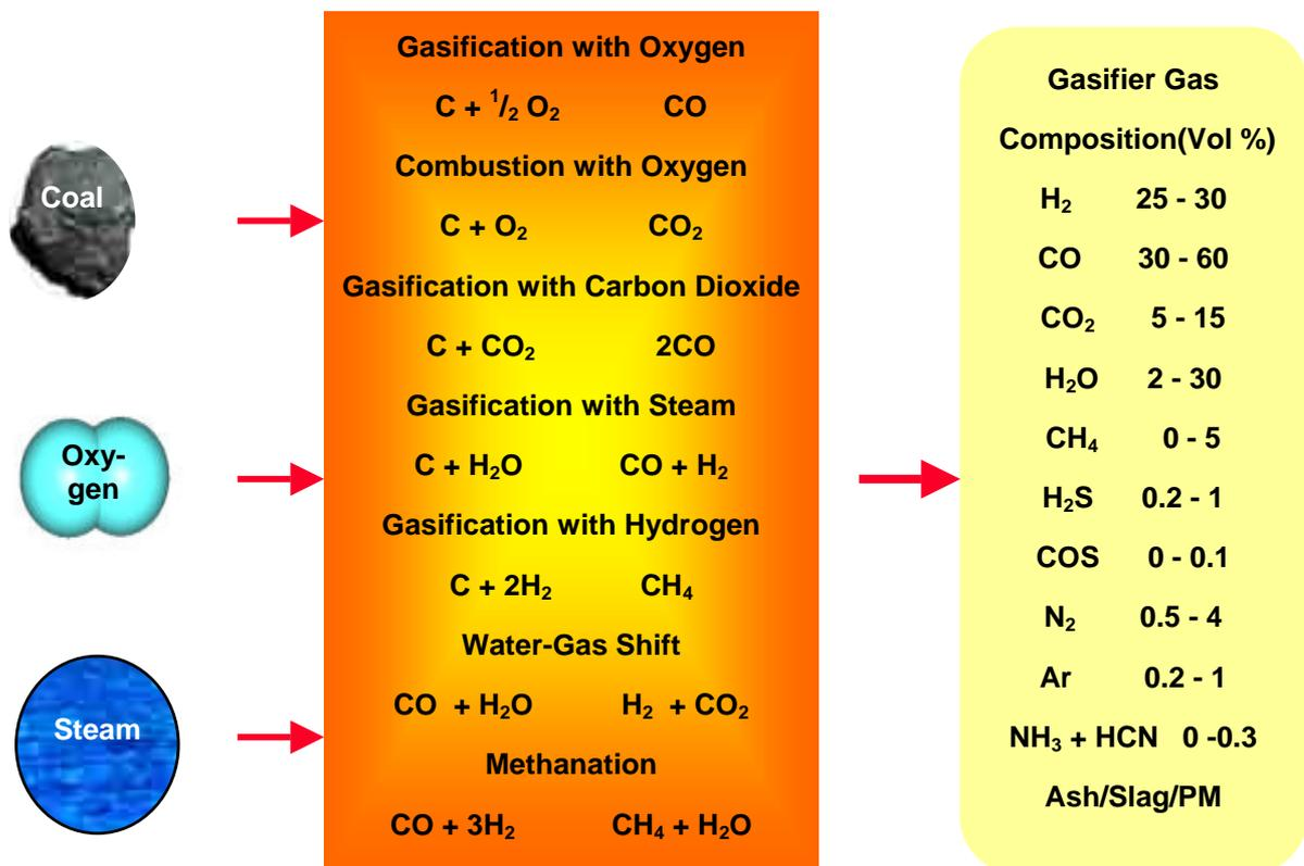
Figure 23: Gasification reaction\_Sengratry/Steve Jenkins\_2007
