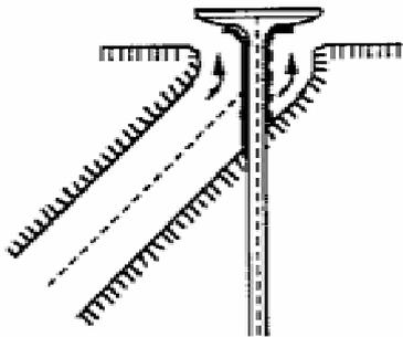
**Figure 31** Tar accumulation on 26 valve and valve stem\_Sengratry/Gary J.Stiegel\_2005
