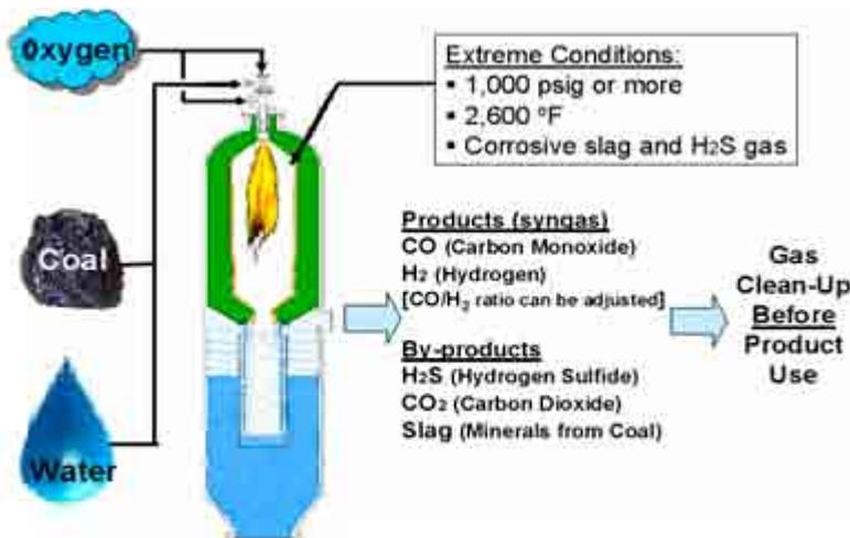
Figure 21: Gasification process\_Sengratry/Gary J.Stiegel\_2005
