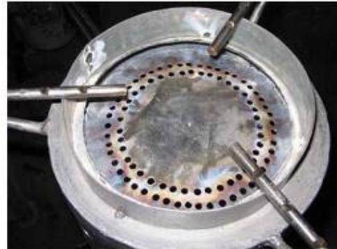
**Figure 12:** The fabricated gas burner\_Sengratry/ Alexis T.Belonio\_2005
