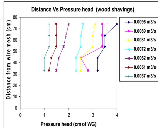
Fig. 7.2 Pressure drop for wood shavings
