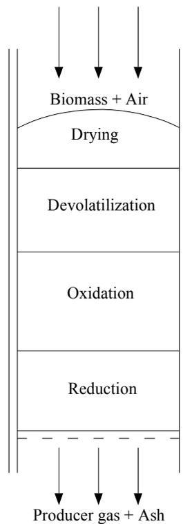
Fig 4.1 Sequence of reactions in downdraft gasifier
