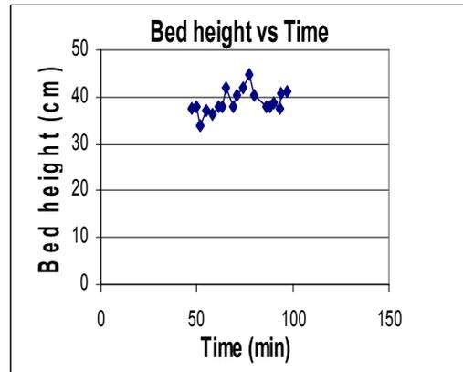
Fig.7.8 Temperature distribution, fuel feeding and bed height change during gasification of wood pieces
