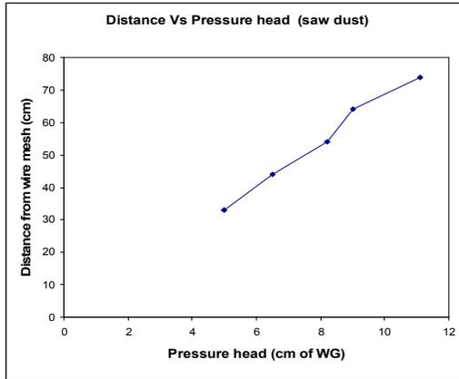
Fig. 7.3 Pressure drop for saw dust
