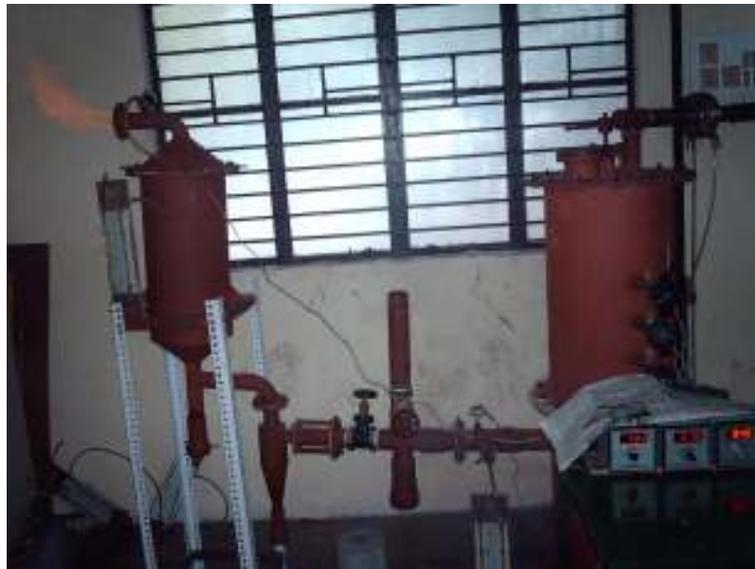
Fig. 6.2 Gasifier in operation
