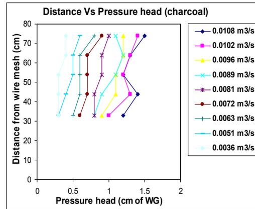
Fig.7.5 Pressure drop for groundnut shells Fig. 7.6 Pressure drop for charcoal
