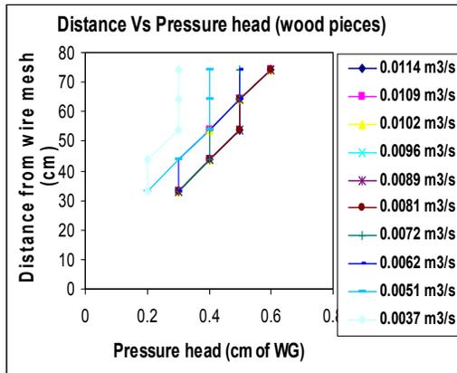
Fig. 7.1 Pressure drop for wood pieces
