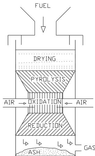
Fig 4.3 Downdraft gasifier
