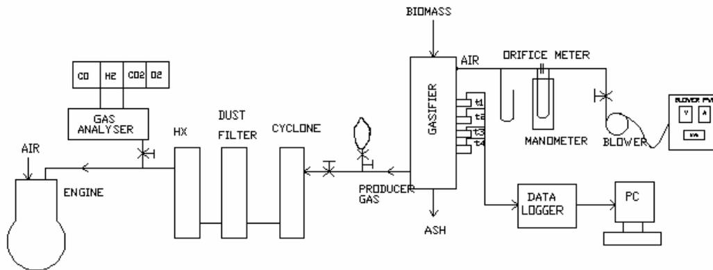
Fig: 5.1 Schematic of biomass gasification system
