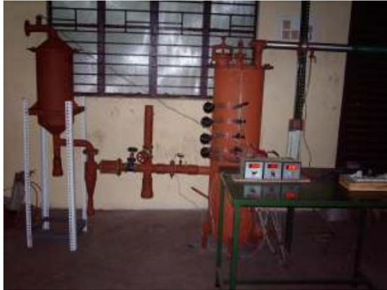
Fig. 5.3 Gasifier for wood and briquettes
