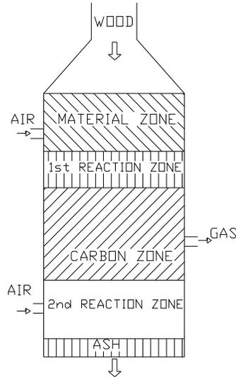
Fig 4.4 Twin-fire gasifier
