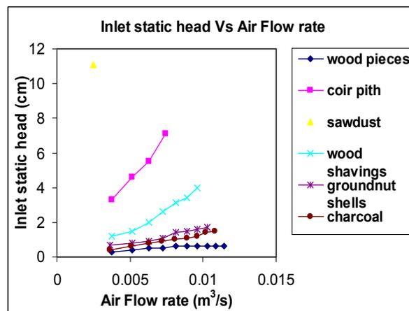
Fig. 7.7 Plot of Inlet static head vs Air flow rate
