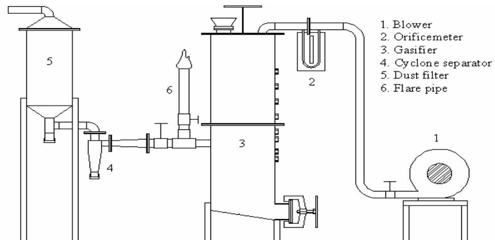
Fig. 5.2 Experimental gasification system
