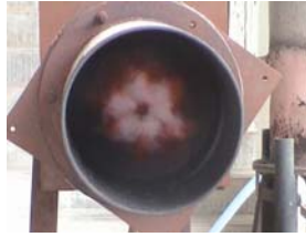
Figure 13: Flame emitted at gas burner with 80mm orifice cylinder and 40° swirler based on the blend of palm oil shell and Mukah-Balingian coal as feed.
