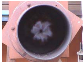
Figure 14: Flame emitted at gas burner with 80mm orifice cylinder and 40° vane based on Mukah-Balingian coal as feed.
